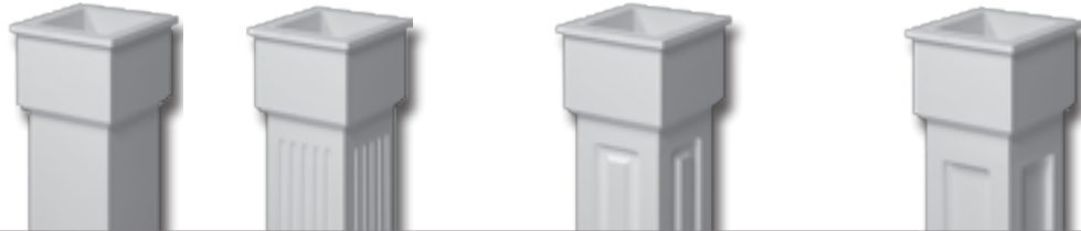
Flutes are 3/4" wide and 3/8" deep. Number and spacing of flutes varies by width of shaft.
